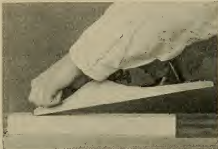
Fig. 38—Lifting Plane on Return Stroke
